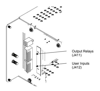
Figure 2.9-1 Interface Connections
